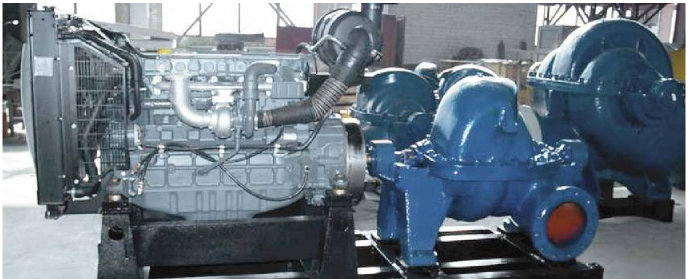
Pump CN 400-105 (Diesel-driven)
